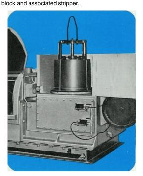
This method of coiling restricts the maximum operating speed and the finishing range of the wire drawing machine. Modern practice is to employ the higher speeds of a capstan type machine with a separate continuous coiling unit. When operated in conjunction with a spooler the coiling block is replaced by a spooling ring.
